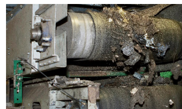
Auto shredder residue being processed over a magnetic head pulley *
